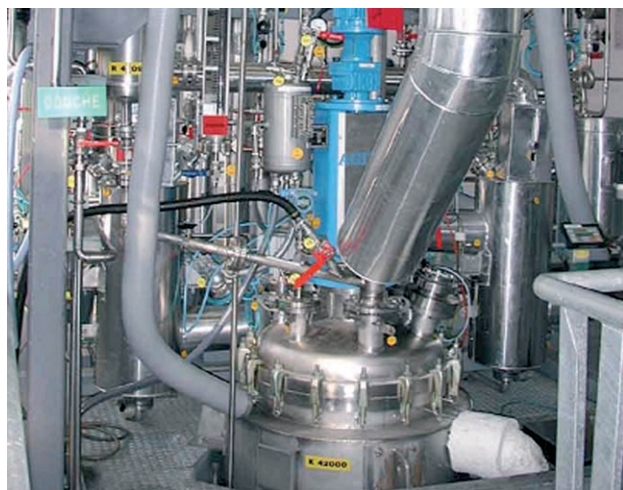
Figure 6. Vessel (250 liters) for the pilot-scale production of A and C .
