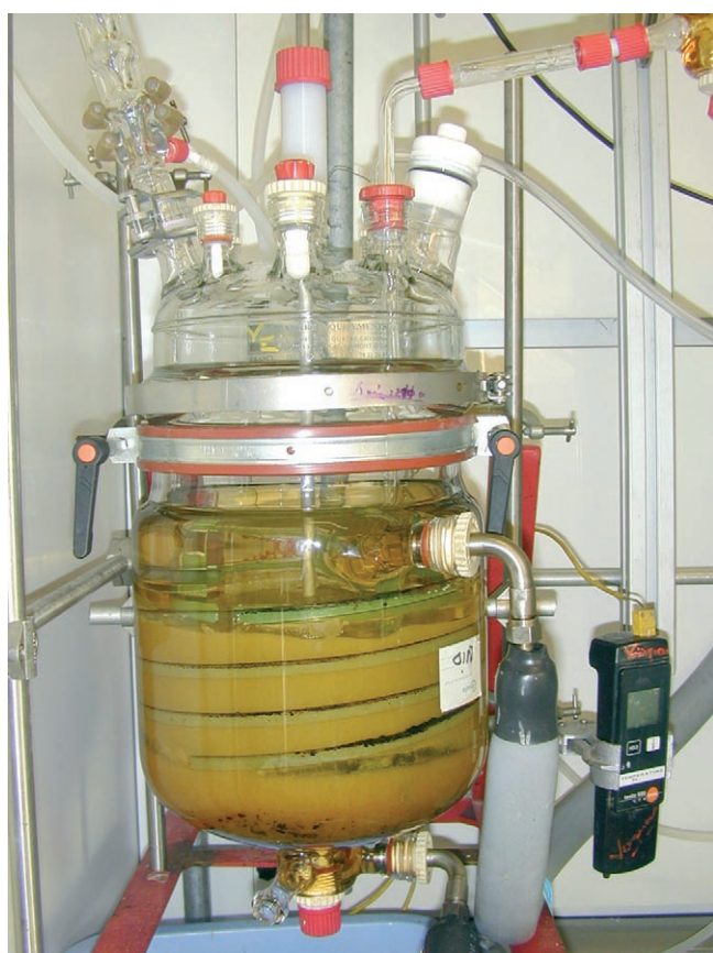
Figure 3. Glass reactor (18 liters) for synthesis of arylhydrazones.
