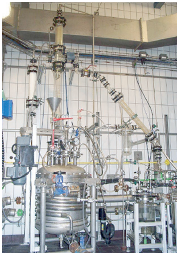
Figure 7. Vessel (150 liters) for the pilot-scale production of B .
