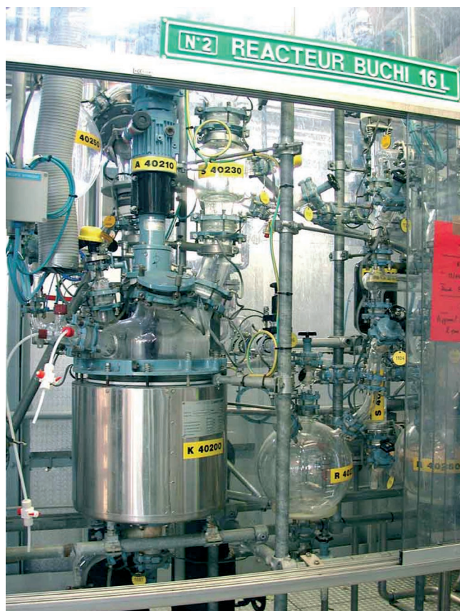
Figure 4. Inox 16-liter Büchi reactor used for hydrolysis of the arylhydrazone.
